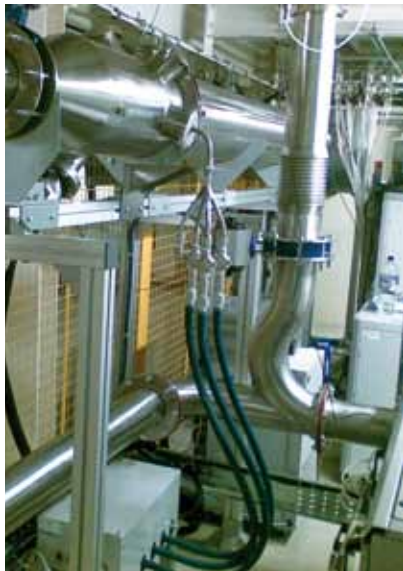
VCA Type approval certified Full flow Duplex particulate tunnel, with 47mm filter holders as per for EU5 requirements.
